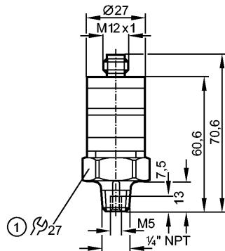
1: tightening torque 25 Nm
